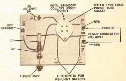
Beginner's one-transistor project uses easy-to-assemble breadboard construction just like the one- and two-tube sets Dad built in the Twenties and early Thirties.
