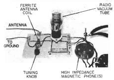
"One tube" receiver uses any old radio vacuum tube (even a burned-out one). Circuit is up-to-date, using hidden diode and transistor.
