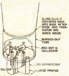
The trick is in the base of the radio vacuum tube. Diode and transistor in its base replace the tube in receiving circuit.
